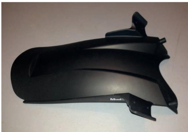
from throwing rocks, tar and debris onto the rear shock, battery, swingarm and surrounding components, areas that are notoriously difficult to access and keep clean. For the purposes of this test, we're using our 2013 R1200R test mule, although Mudslings are available for a variety of different BMW's (including GSs!).
