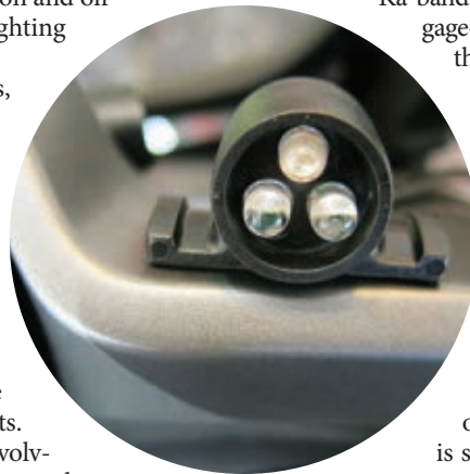
The Visual Alert 3/4-inch LED array fit easily on the R1200RT's dashboard.
