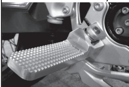
High traction footpegs for the R9T and other BMW models. 1.2" lower than stock.
