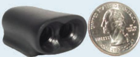
uses the air pressure at the front of your vehicle to produce an audible, forward-facing tone “alert.” In its favor, I can say that I hear the whistle at speeds of approximately 50 MPH and above. If I’m riding into the wind, I can sometimes hear it at 40 MPH, but if I have a tailwind, I don’t hear it until I reach 60 MPH or better.
