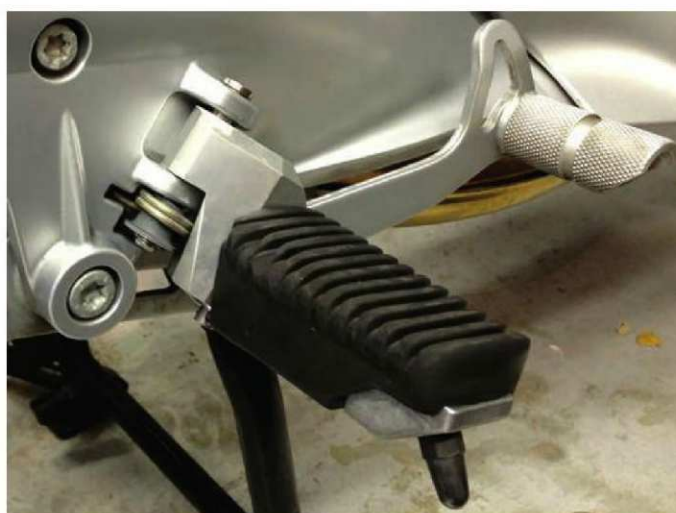
Figure 4: Suburban Machinery footpeg lowering brackets installed – move stock footpeg location 1.45” down and 0.38” forward.
