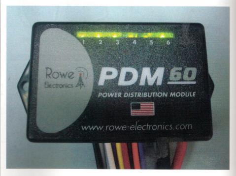
settings such as circuit behavior mode (inactive, live, trigger, and so on), current limit for each circuit and delay on/off settings.
