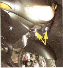
be drilled where the Bullet light is to be mounted, to allow the wires to pass through. On some applications, like the RT location shown here, this is not an issue since the holes are hidden. But other potential locations exist where owners may be less than anxious to drill. Fortunately, BikeVis tells us that Bullet lights with the wires routed out of the rear of the housings should be available soon.
