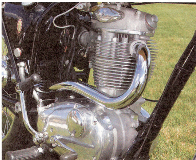
Above: The Victor's "round barrel" 441cc single was actually based on BSA's 250cc cases. The compact unit made 30hp.
