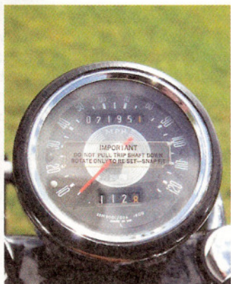
Above Left: The Victor's 32mm Amal carburetor. The brass plunger in the center is the "tickler" or starting enrichener. Above Right: Smiths speedometer also featured a tripmeter.
