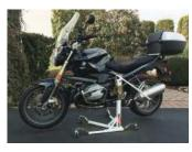
Using the Bursig is a one-handed affair, with the entire operation taking place right next to the bike, instead of behind it, as with conventional swingarm stands. Better yet, once hoisted, any manner of service is possible, since the stand doesn't block many major components from being removed. It's a one-person operation, with leverage provided by the handle that enables easy lifting and lowering.
