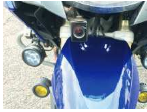
The K1 video recording system by Innovv includes two cameras, one for front mount (left) and one for rear (right). The DVR control module is not waterproof and must be mounted in a weather-protected part of the bike, which may be inconvenient.
