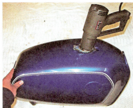
Left: Corks from the local hardware store are perfect for plugging the tank bungs. Center: Duct tape works well to seal the tank's filler hole. Right: Use a heat gun to completely dry the tank prior to application of the final sealer—this is critical.
