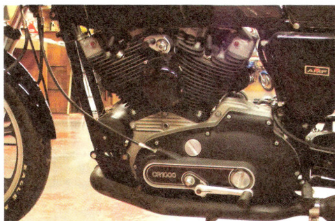
Above: The left side reveals the XLCR’s iron cylinder barrels. Inside the cases was a high-effort four-speed transmission.
