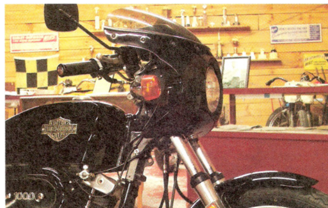
Above: The XLCR’s bikini fairing was a fairly generic design, similar to what you’d get with a Ducati or BMW, but it gave the machine a sportbike style like no Harley-Davidson before it.
