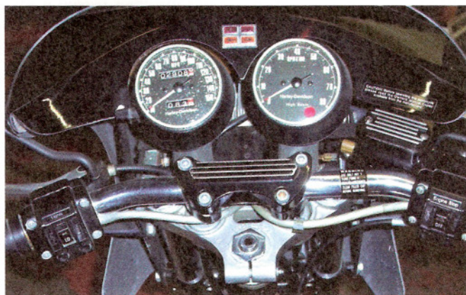
Above: The speedo and tachometer were the same style as used by Honda at the time and marked with optimistic numbers: The top speed, 150 mph and the tach to 8000 rpm!
