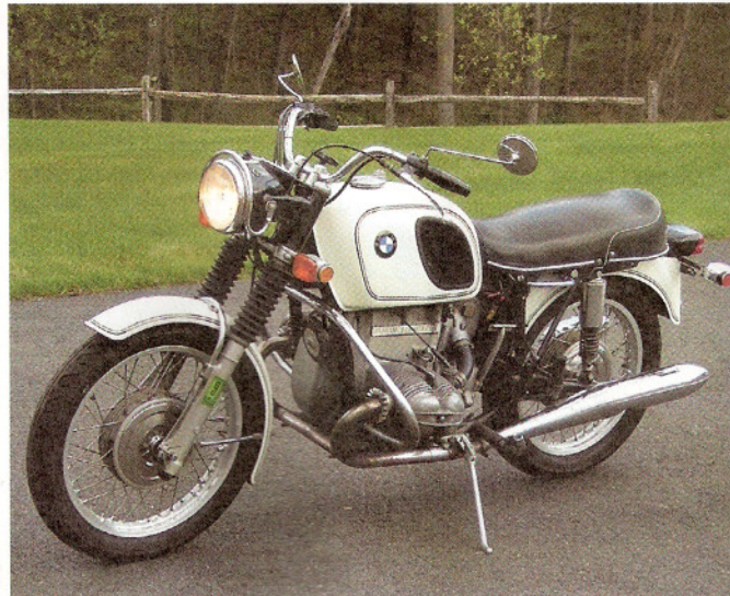
The author's wife's first bike, a 1971 R60/5 with standard 6.3-gal. tank. With almost 100,000 miles, it's still going strong.
