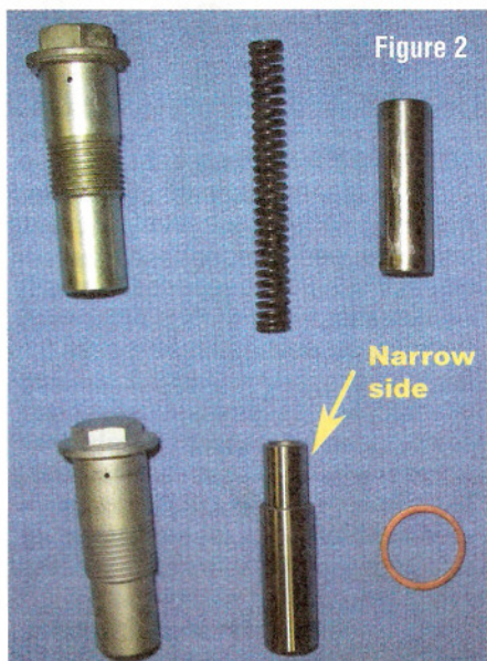
Original Oilhead Tensioner Assembly on top vs. new kit below.
