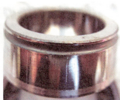
(Fig. 6) This OEM bearing race displays the ravages of hard use. Left unchecked, the bearings could've seriously affected driveline stability.
