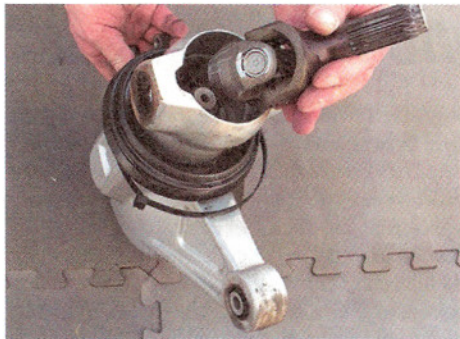
(Fig. 4) Removing the housing exposes the offending OEM needle bearings. It is important to do the work on a non-marring surface to protect the paint on the housing.
