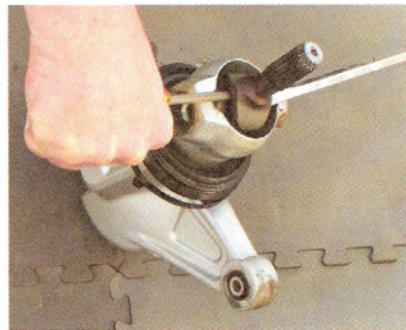
(Fig. 3) Once the final drive is removed, it can be placed on a flat surface and the U-joint can be extracted from the housing with a pair of flat-blade screwdrivers.
