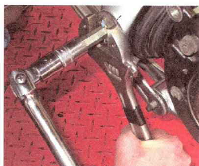
(Fig. 12) Reinstall the final drive, adjust U-joint freeplay with the adjustable pivot pin and tighten both pivot pin locknuts. Then rejoice, the hard part is over!
