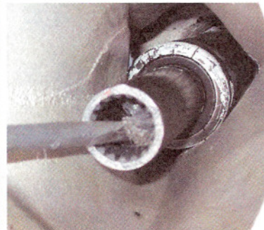
(Fig. 9) Apply moly paste to the bearing races (bushing OD) and to the driveshaft splines (shown), but don't apply any to the bushing ID.
