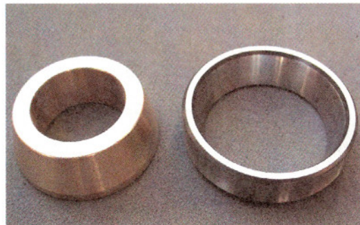
(Fig. 7) Beauty that is beyond skin deep: The JL bushing kit replaces the OEM needle bearings with self-lubricating bronze bushings (left) and high-quality Timken bearing races.
