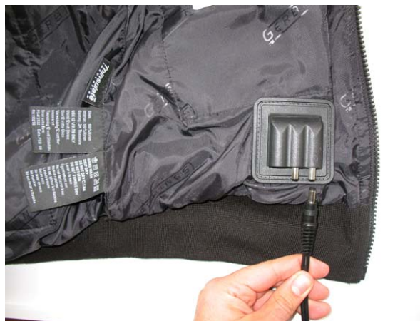
Figure 8: Gerbing's PDU has three connections: White-tip plug closest to the zipper is main input, middle plug is for separate glove control (if desired,) and outside plug can be used for additional garments.
