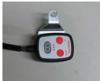
Figure 16 Caption: Stormrider Controller measures approx. 1”H x 2.3”L x 1.8”D (not including the bracket).
