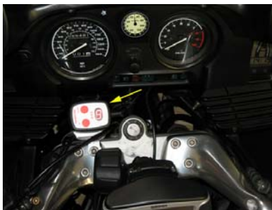
Figure 18 - EXO 2 Stormrider controller mounts perfectly on BMW RT test mule using existing handlebar hardware.
