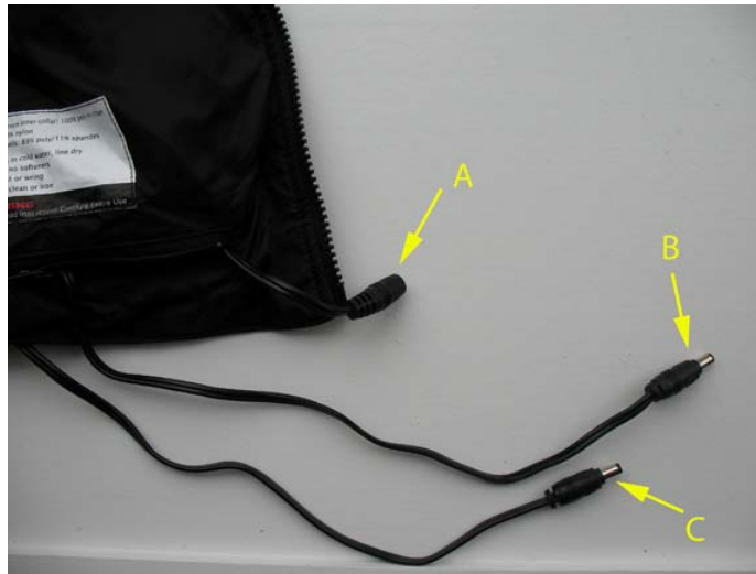
Figure 5: FGWNS coax connectors. A is for additional garments, B is for separate glove control, and C is main liner power input. All store in dedicated pockets within the liner.
