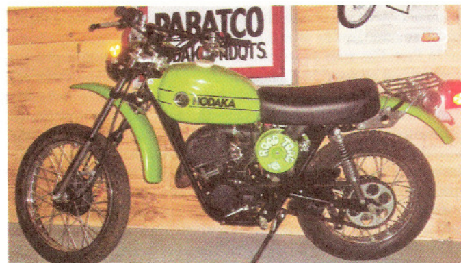
The 100cc Road Toad was typical of the lightweight two-stroke "enduro" (dual-purpose) motorcycles of the 1970s.
