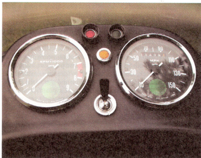
Classically elegant Smiths gauges dominate the JPS' instrument panel. Idiot lights are for ignition, t/s and high-beam.
