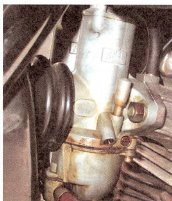
Left: The John Player Special's large bug-eye headlights were a distinctive feature of its fairing design. Center: Dual 32mm Amal "carburetors," a British standard, feed the Norton twin. While it may have more in common with a Commando than a Norton factory racer, the John Player Special is an esteemed British classic, with examples selling for as much as $15,000 today.
