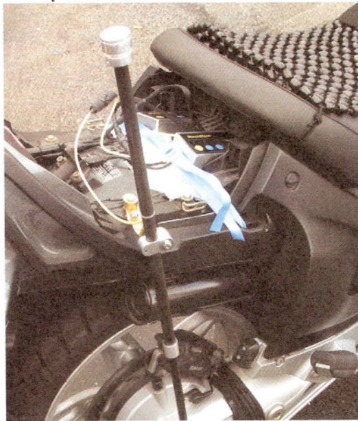
Left: Front ShockClock Transducer mounted on the RT's handlebar. Middle: Rear ShockClock Transducer fully mounted with Data Recorders secured in place of the RT's passenger seat. Right: An example of a construction road used in Test 3.
