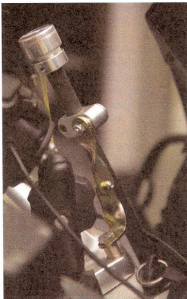
Left: Front ShockClock Transducer mounted on the RT's handlebar. Middle: Rear ShockClock Transducer fully mounted with Data Recorders secured in place of the RT's passenger seat. Right: An example of a construction road used in Test 3.
