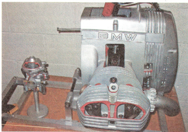
Bing Carburetor and BMW Airhead Engine cutaways at Airhead Supertech 2009. Props like these can be invaluable for educating Tech Day participants on DIY service issues.
