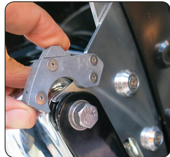
Included Trigger Lock latching mechanisms are made of glass-filled nylon, for strength and light weight
