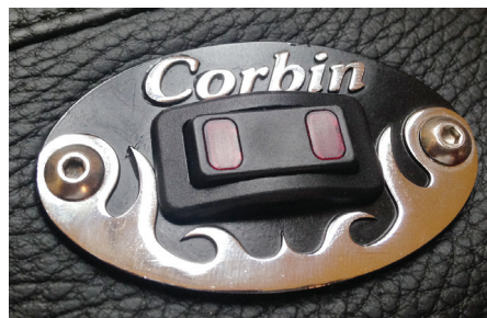
Illuminated three-position rocker switch controls the heat settings on the seat
